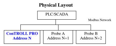
The Controller will pass through any messages sent between the SCADA/PLC and Probe A or B. The Controller must also poll the probes for measured values to control the analog outputs, relays and internal log as well as the local display. When the Controller is polling the probes for measured values, the SCADA/PLC will get a modbus exception 0x06 (slave device busy).
