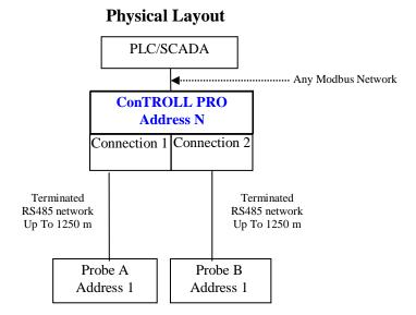
The Controller will have a contiguous address block associated with it that begins at the controller's assigned device address and ends at the controller's device address plus the maximum number of connections supported by the controller. The Controller will always occupy the same number of contiguous addresses regardless of the number of probes actually connected.
