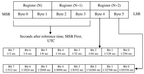
**Time Example:** For a time value of 0x001A5E00C000, the bytes 0x001A5E00 represent the whole number of seconds from the reference time. The bytes 0xC000 represent the additional fractional number of seconds as shown in the diagram above. In this example, the whole number of seconds represents 20 days and the fractional seconds represents 750ms.
