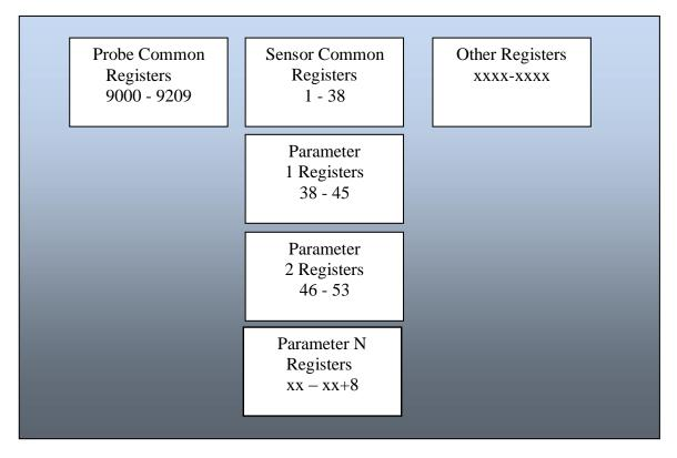
All registers in this document are 1-based. This means the actual packets sent to the devices must have a data address 1 less than what the register number is in this document.
